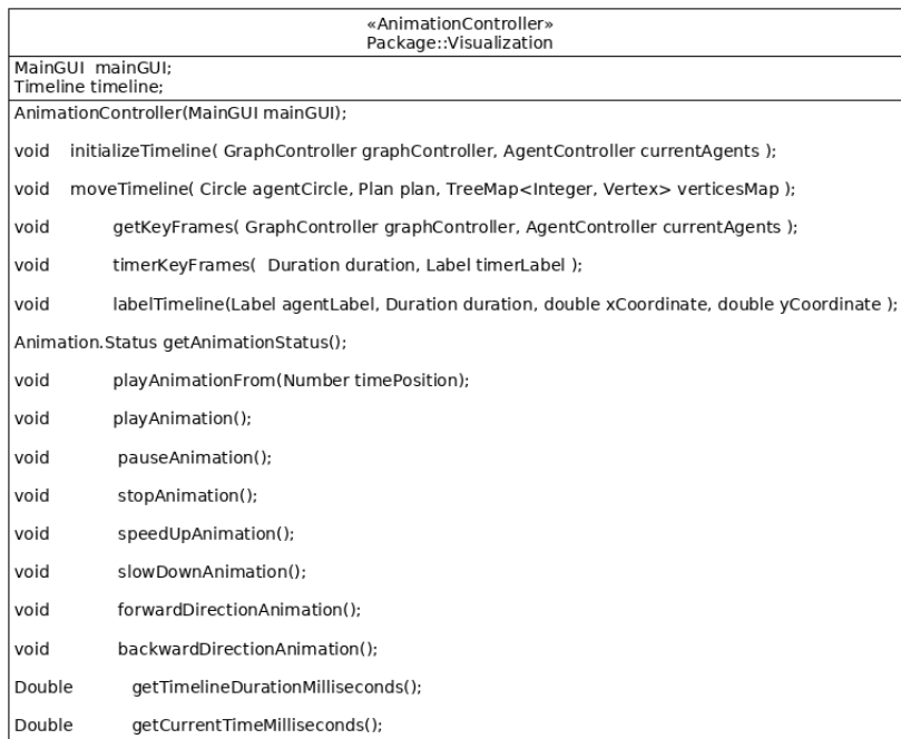
Figure B.4: b. Visualization module class diagram
