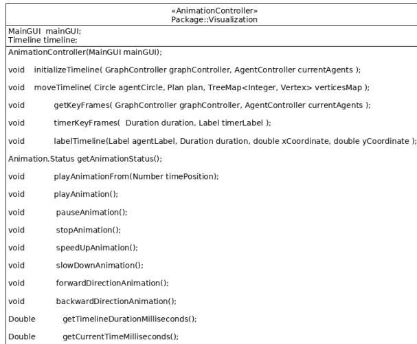
Figure 3.4: b. Visualization module class diagram
