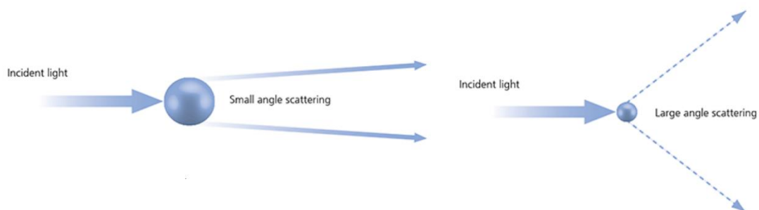
Figure 41: Light scattering in laser diffraction measuring method for larger and smaller particles [74]
