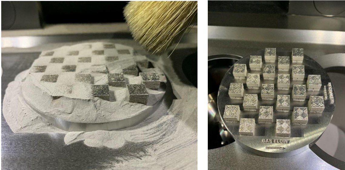
Figure 56: Final printed L-40 platform for 200 W – on the left de-powdering, on the left finished platform
