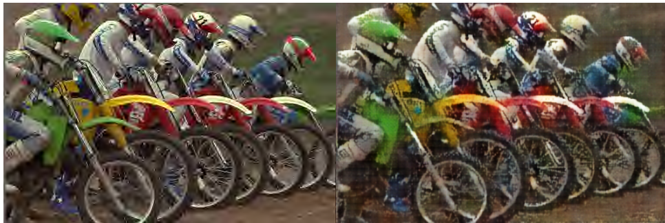
Figure 3.1: Comparison of (left) conventional compression method JPEG2000 (right) ML-based compression system [50] with identical target compress ratio of 192 : 1 (0.125 bpp)
