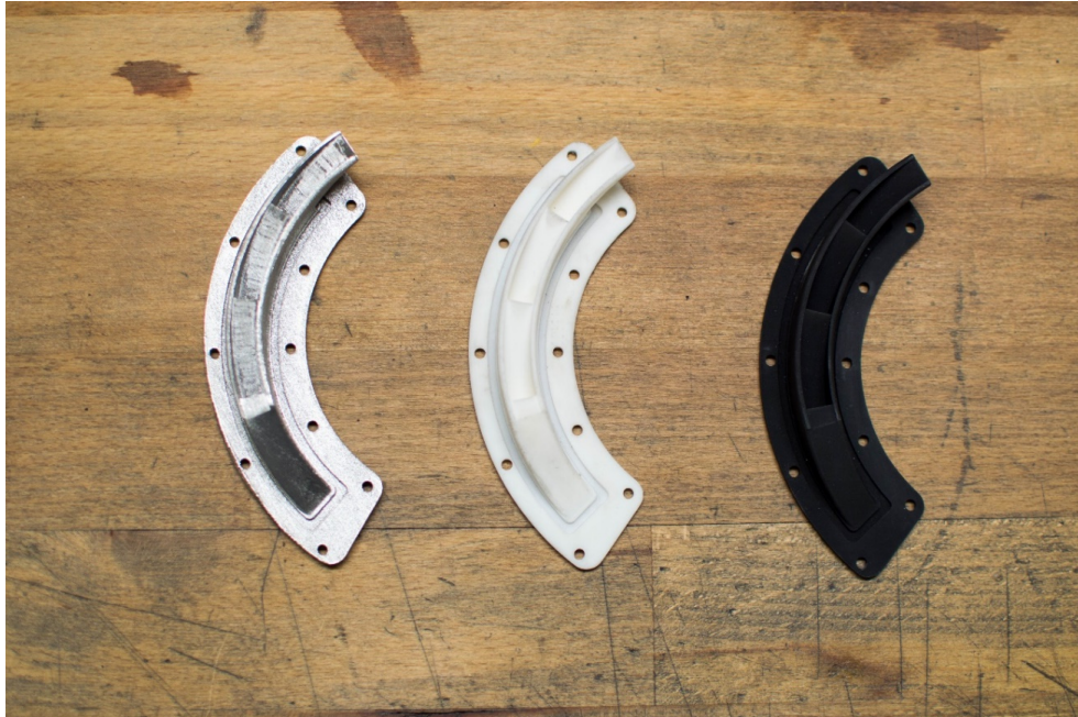
Figure 5.5: Experimentally investigated nozzle segments made of different materials by different AM methods; from left to right: DMLS stainless steel, SLS nylon, SLA resin
