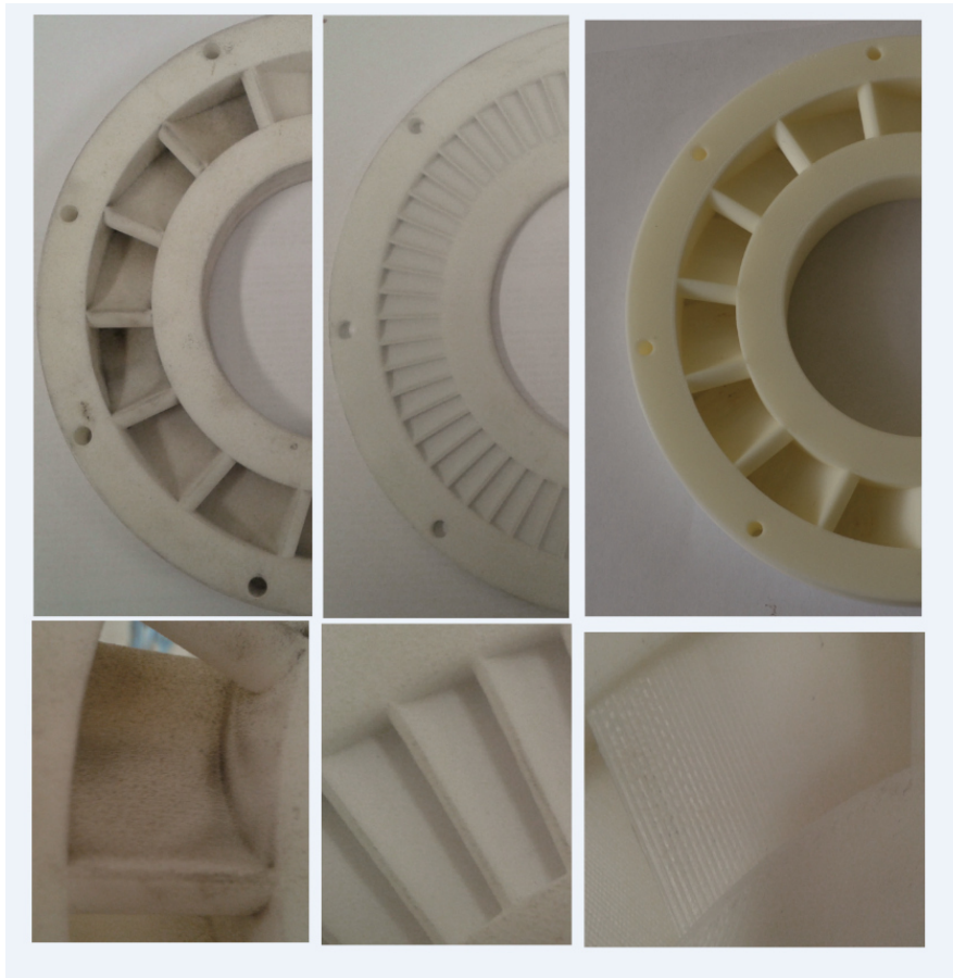
Figure 5.3: Experimentally tried stator wheels; from the left – SLS long chord, SLS short chord, FDM long chord
