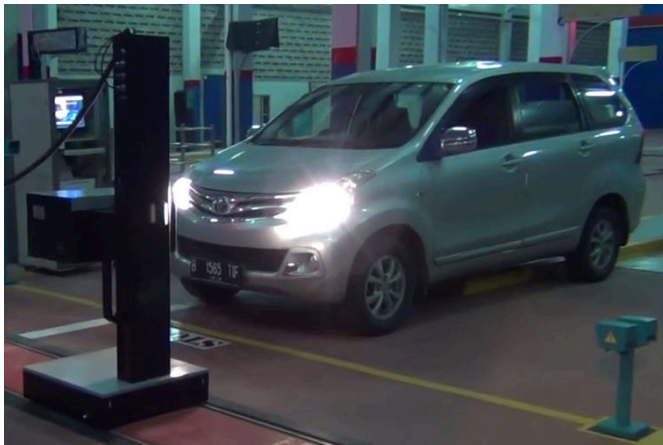
(a) : The headlight tester in use.
