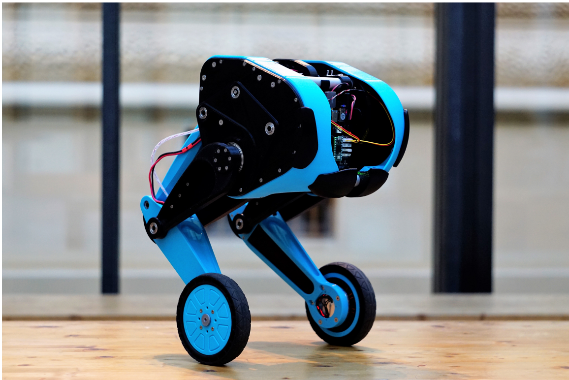
Figure 1.1: First working prototype of our bipedal wheeled robot.
