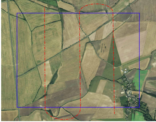
(a) A depiction of the scanning phase of the area coverage with a draft of possible coverage trajectory (red) to detect regions of interest.
