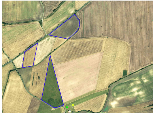
Figure 6.6: The third experimental scenario. The regions to be covered (blue polygon) represents two fields that are close to the starting point (yellow dot) and the ending point (green dot.)
