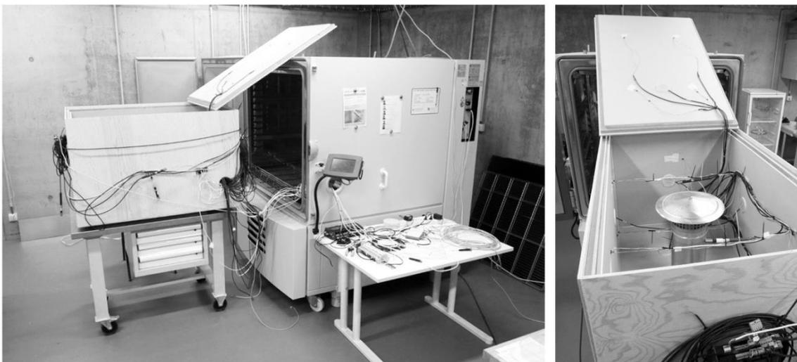
Fig. 21: left: test box in front of climatic chamber; right: open test box with hygro-thermal sensors and heat source
