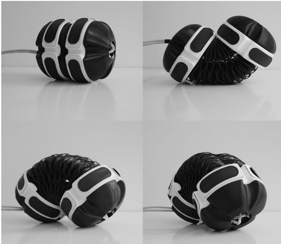
Fig. 64. Bending in different directions by synchronisation of the vacuum and compression in Version 3.
