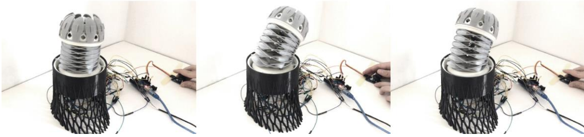
Fig. 42. Mole Version 1 and its bending in all four directions.
