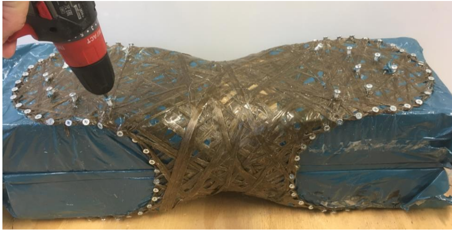
Fig. 53. MoleCHAIN passive part created by winding flax natural fibre around a mould.
