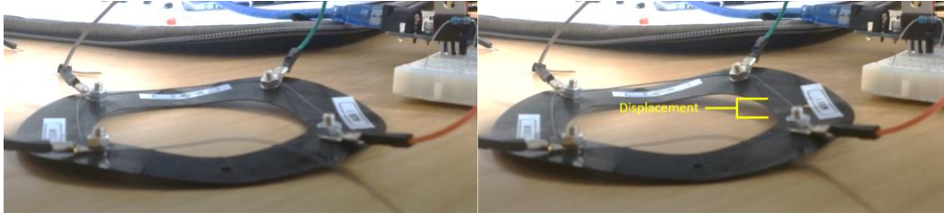
Fig. 34. Testing of Flexinol® for Mole soft body within the MoleMOD system.
