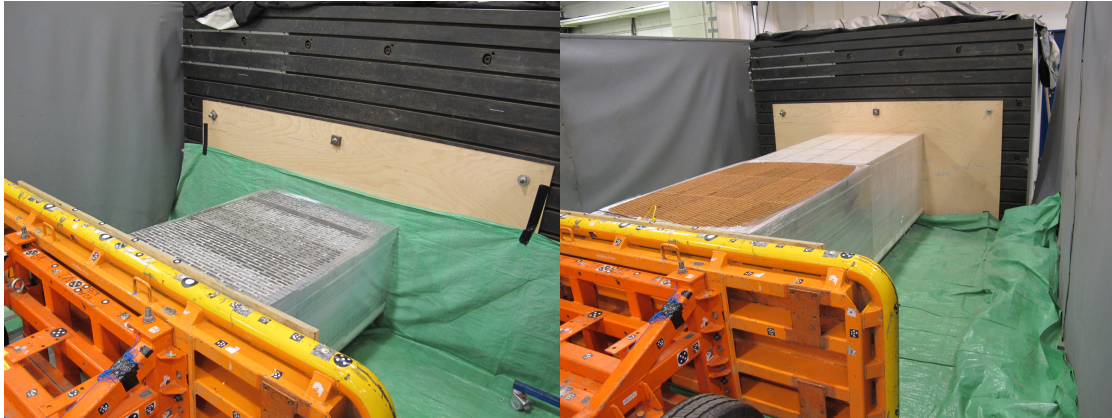
(a) Collision with a crash cushion made of high-performance concrete.
