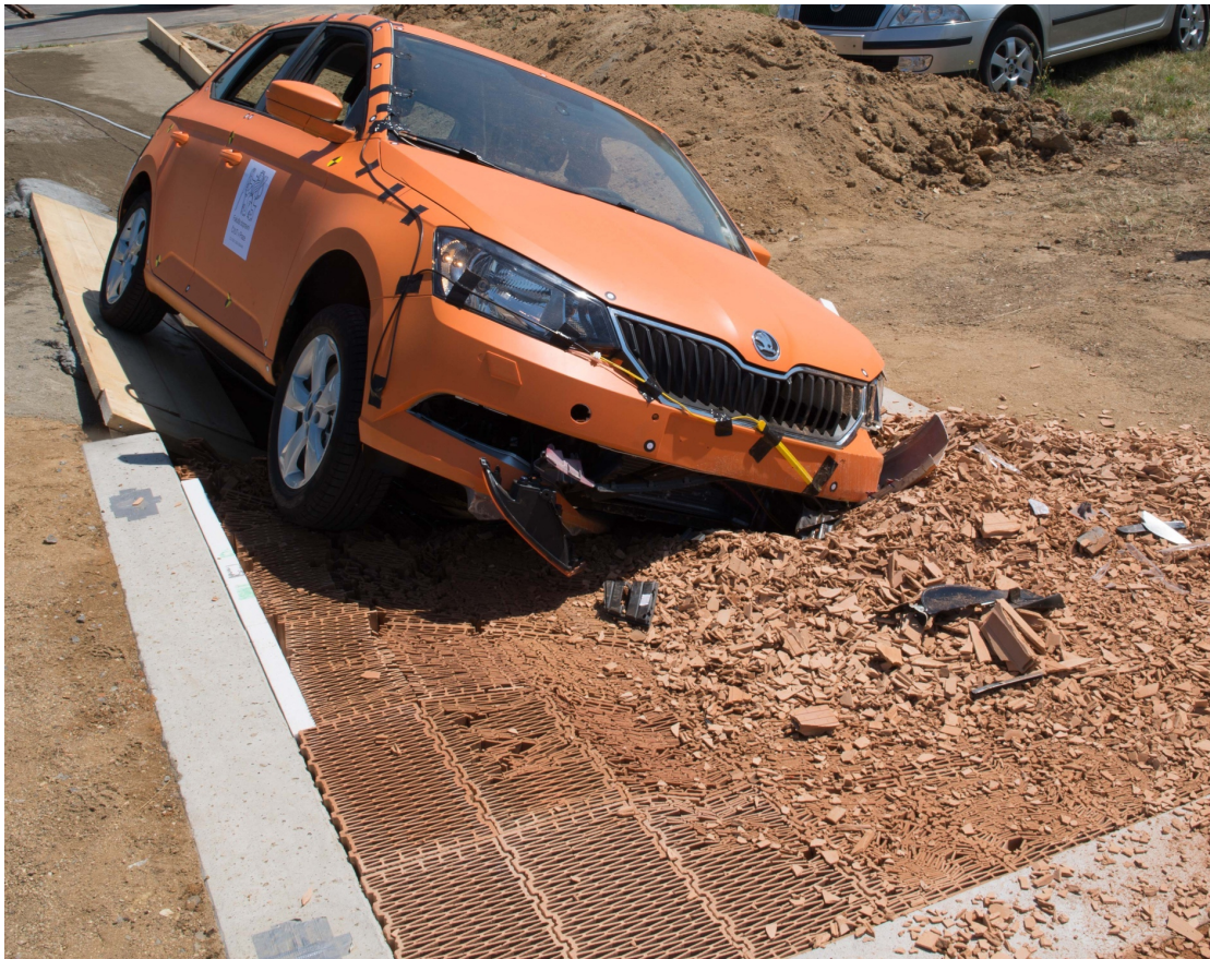
Figure 3.1: A passenger vehicle after impacting the novel energy absorbing system comprised of brittle blocks with thin-walled cellular structures.
