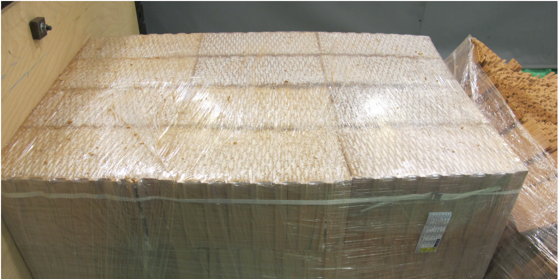
Figure 2.9: Semi-stiff part of specimen after 34.7 kJ impact.
