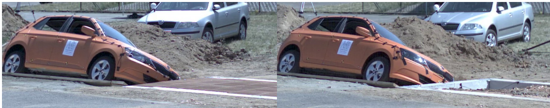
(a) Collision with a crash cushion made of fired clay.
