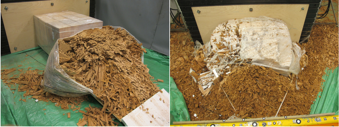
Figure 2.8: Soft and semi-stiff part of specimen after 34.7 kJ impact (left) and 96.5 kJ impacts (right).
