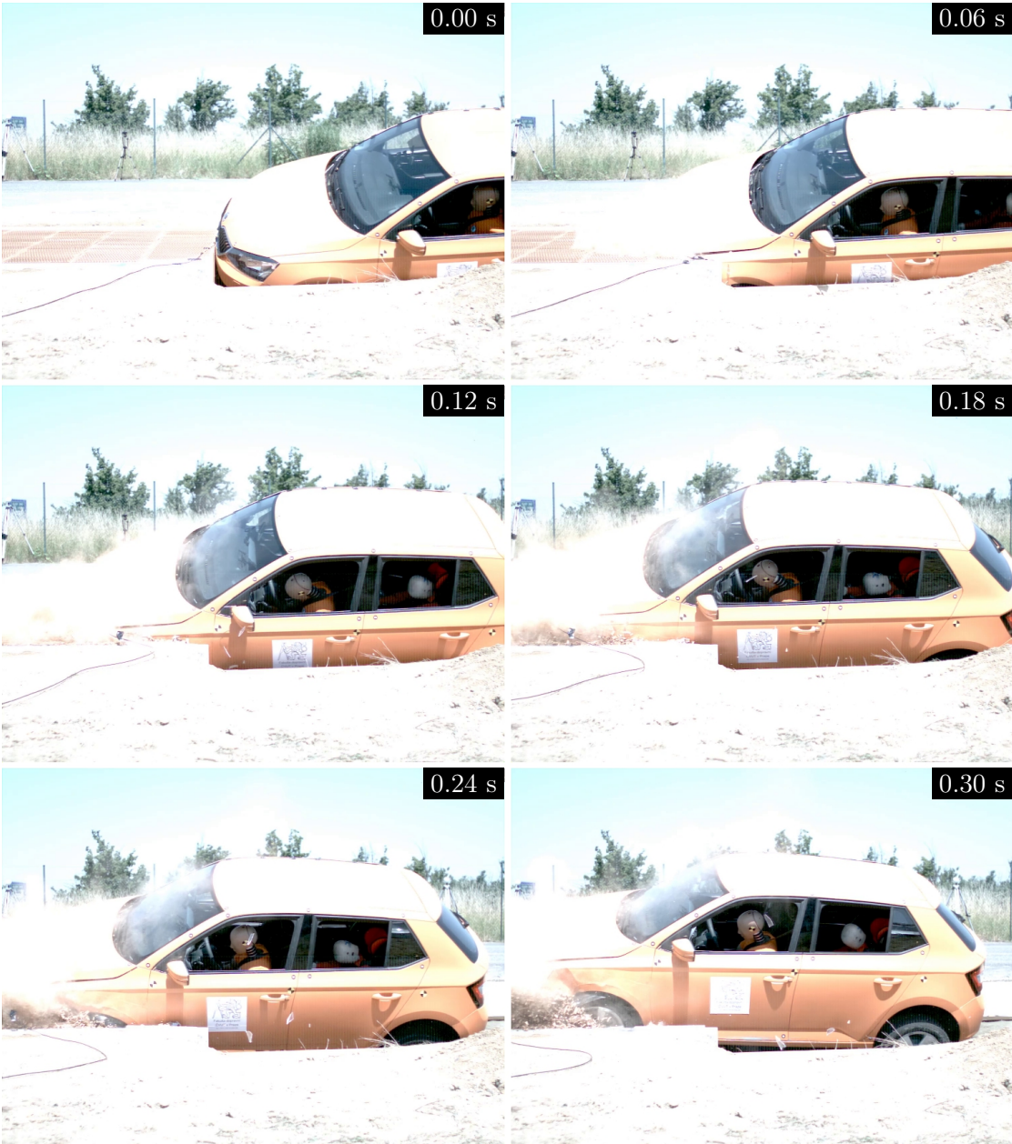
Figure 2.17: Collision of Skoda Fabia vehicle with deformable specimen of trimmed bricks with cellular structures.
