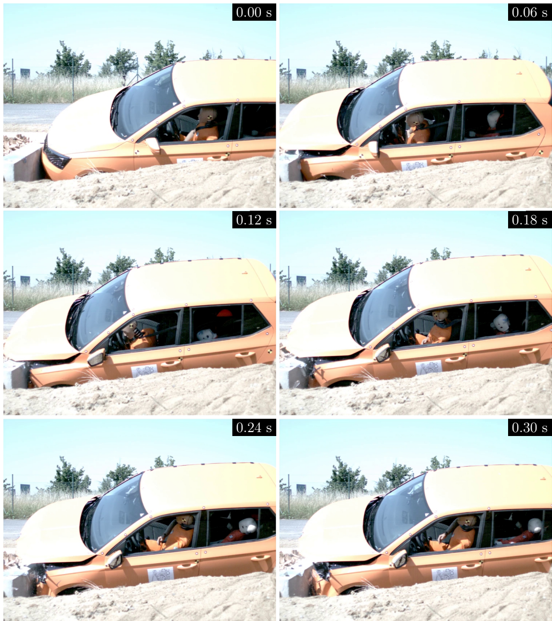
Figure 2.16: Collision of Skoda Fabia vehicle with non-deformable reinforced concrete specimen.
