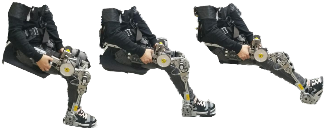
Figure 4.25: Exoskeleton aided leg rise on a human subject.
