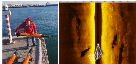
Fig. 2. LAUV vehicles being deployed for the experiment (left) and sidescan data acquired (right)
