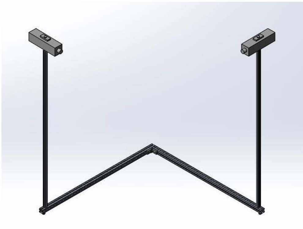
Figure 10 Lightweight aluminium construction that ensure the correct camera positioning.
