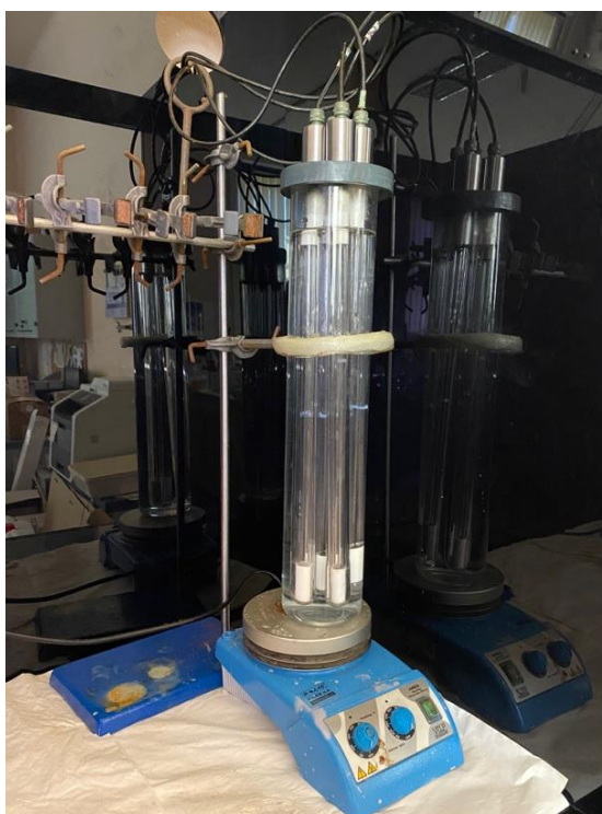
Fig. 20: Photochemical set-up for irradiation using low-pressure mercury lamps.
