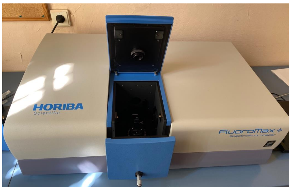
Fig. 19: Horiba Jobin Yvon FluoroMax4 spectrofluorometer.
