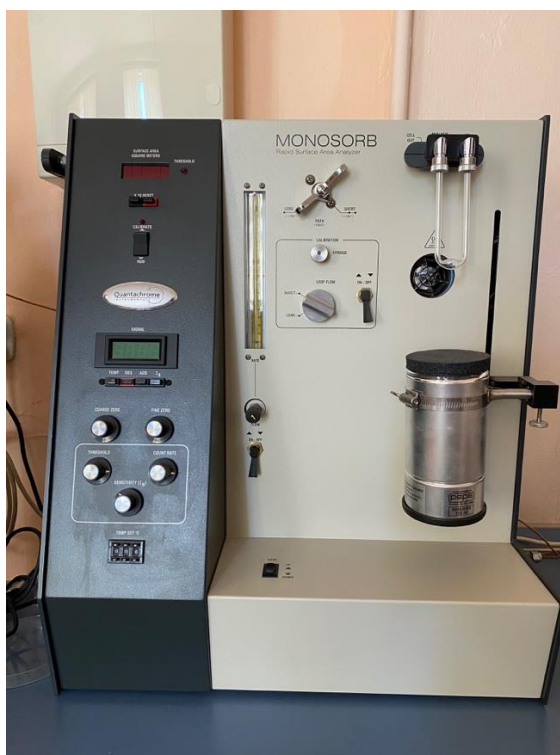
Fig. 17: Monosorb MS-22 surface area analyzer.
