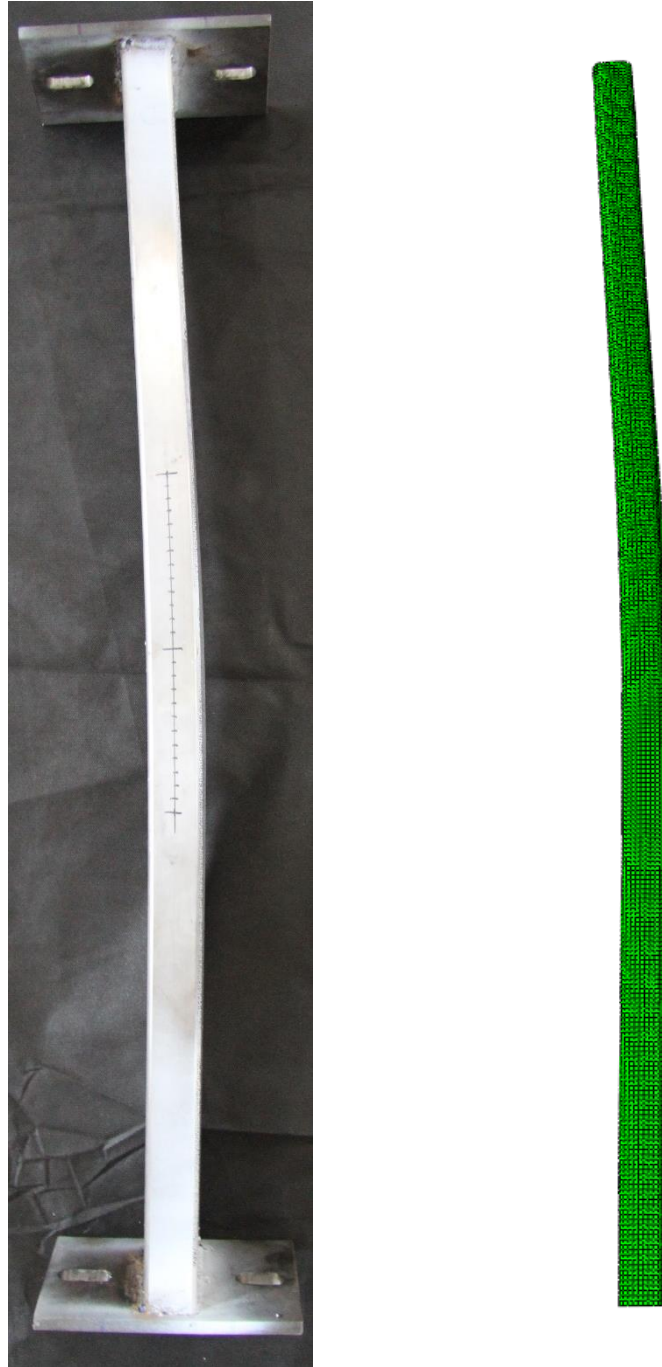
Figure 5.11 Test and numerical minor axis flexural buckling failure of specimen 17.
