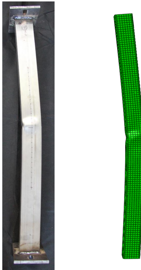
Figure 5.9 Test and numerical local buckling failure of specimen 13.
