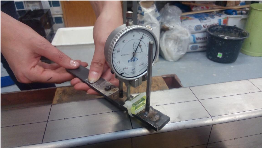
Figure 4.9 Local imperfection measurement.
