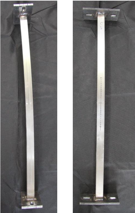
Figure 4.17 Flexural buckling failure.
