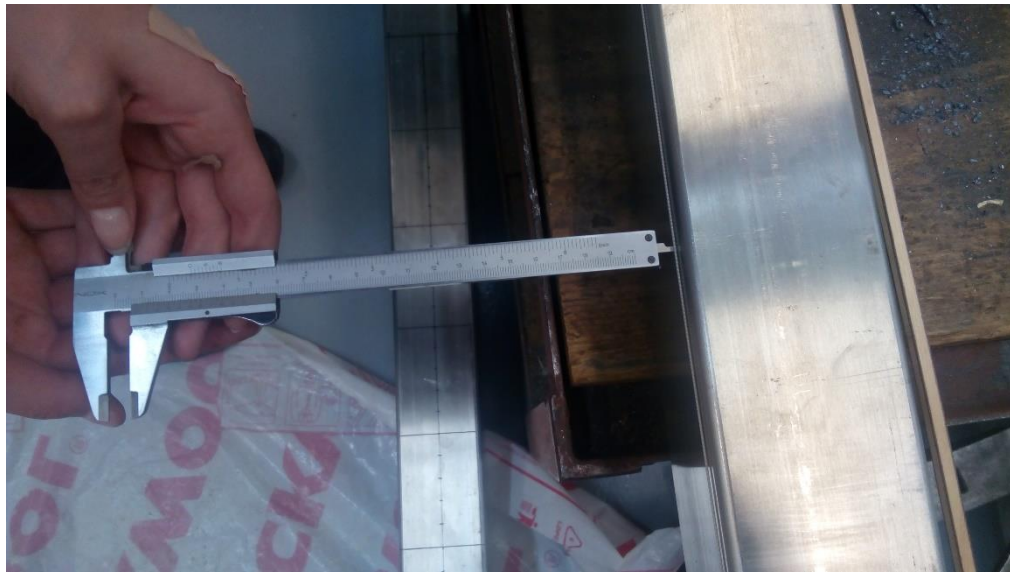
Figure 4.7 Global imperfection measurement.
