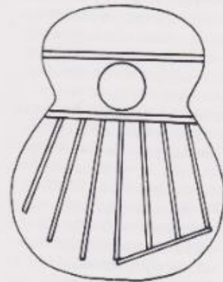
7-3. Asymmetrical variations of the classical soundboard.
