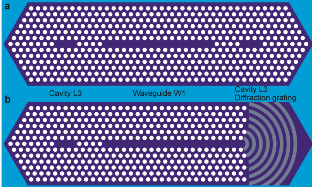
Figure 22: Sketch of the simple integrated photonic structures: (a) Two L3 PhC cavities coupled via W1 PhC waveguide. (b) L3 PhC cavity coupled to W1 PhC waveguide, and periodic diffractive grating for Bragg diffraction of light from the slab plane into the space.
