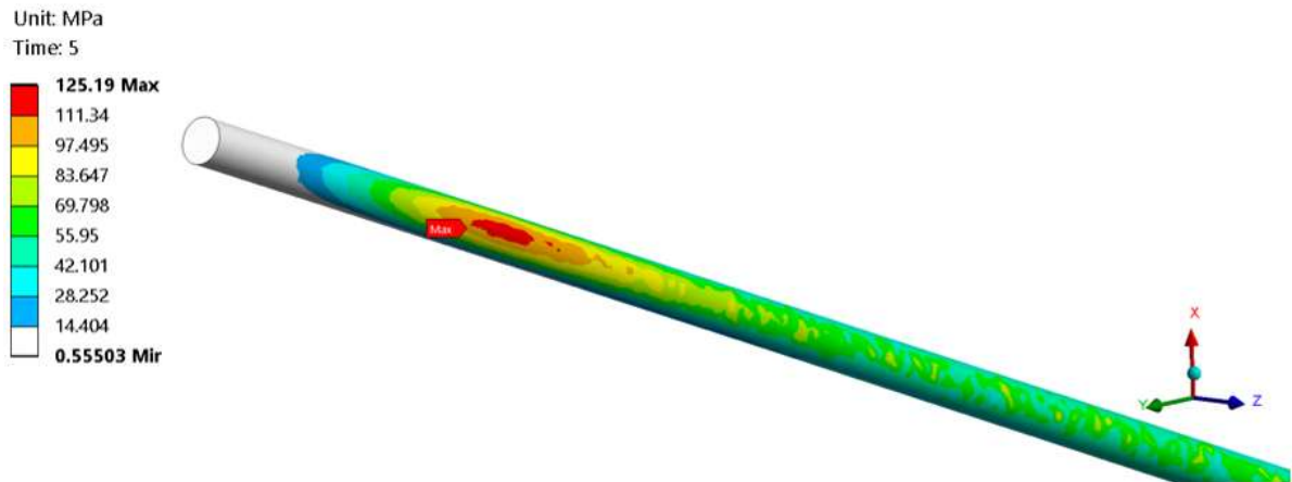
Figure 62. von-Mises stress in GRIN -lens surface, MR.c (125.19 MPa).
