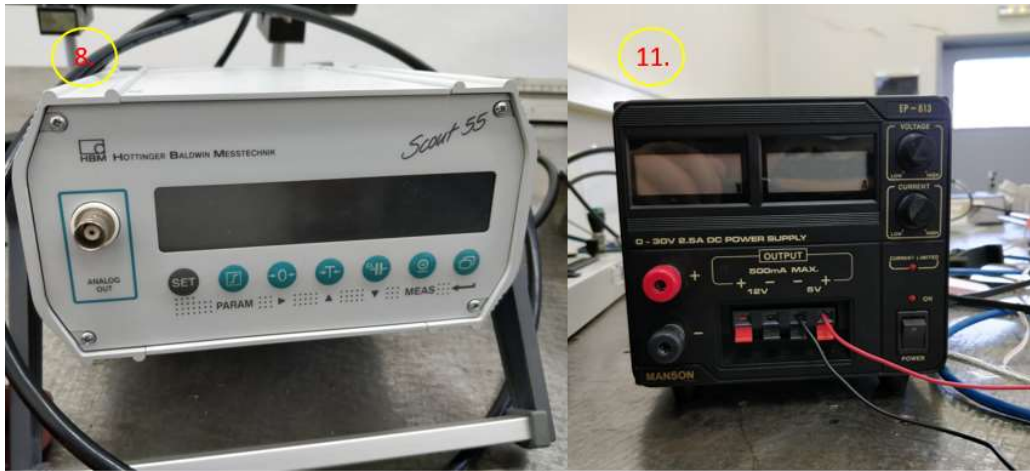
Figure 41. Amplifier and power source used in the experiment.
