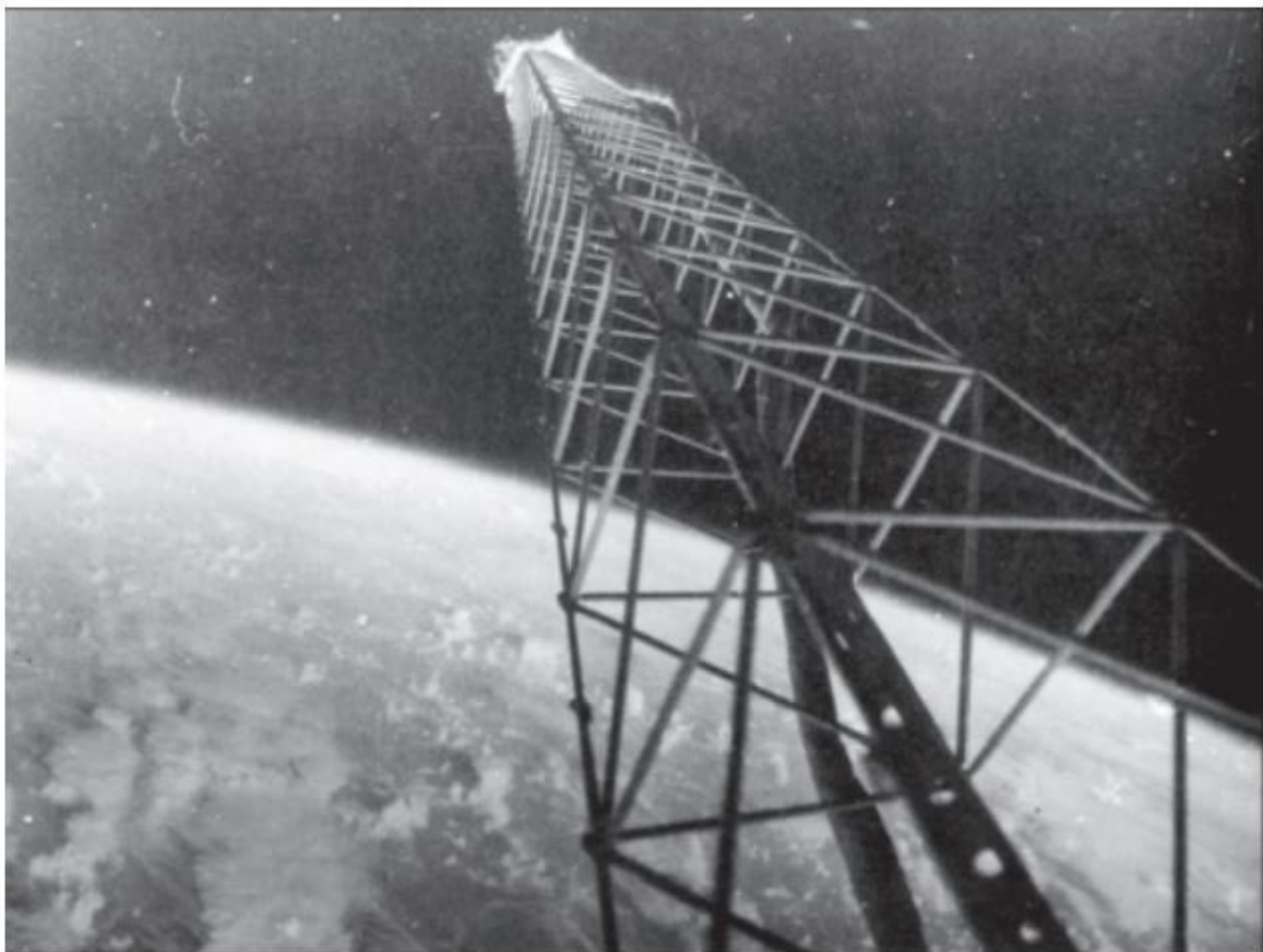
Figure 3 - Truss mast Mayak in its deployed state [2]
