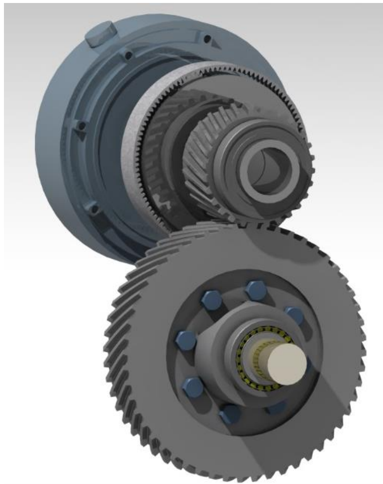
Fig. 65 The Planetary Gearbox For Electric Vehicle in CATIA V5
