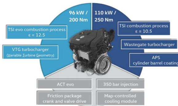
Figure 11 - Variants and technologies EA211 1.5l TSI evo [14]
