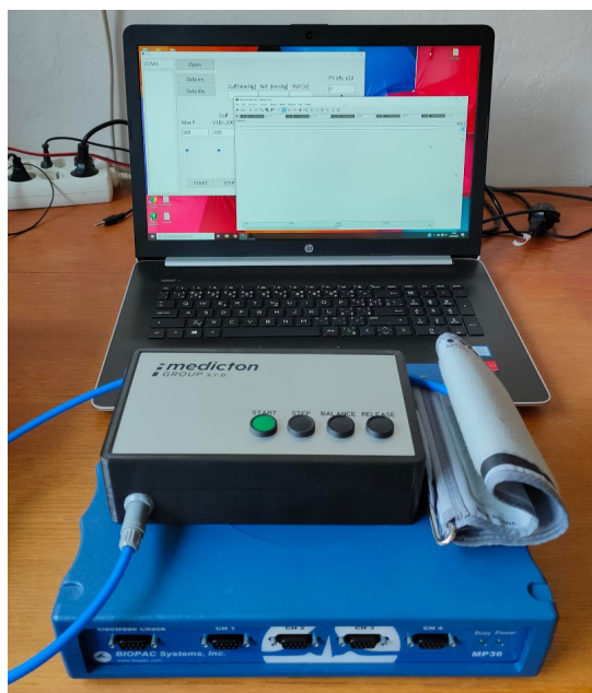
Figure 40: The PWV measuring system using BIOPAC from step four
