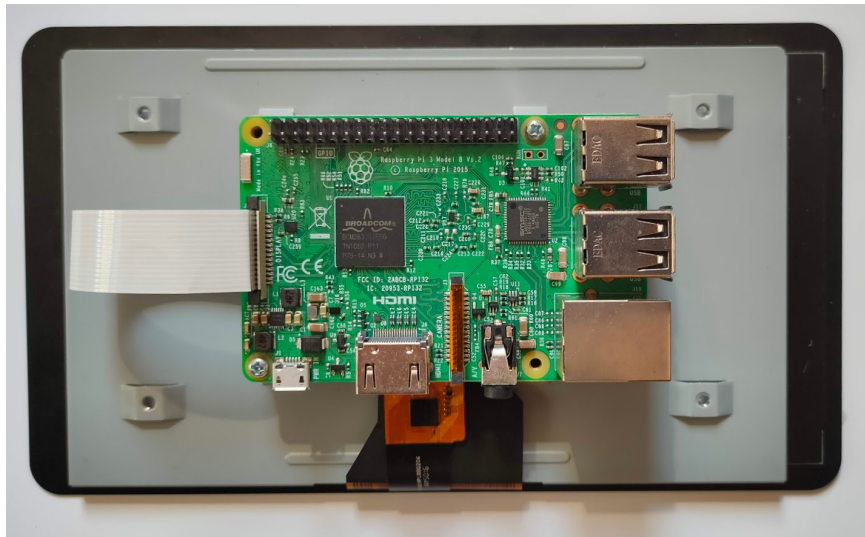
Figure 18: Raspberry Pi mounted on the back of the touchscreen
