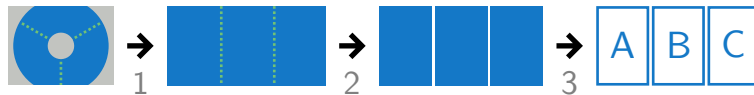
Figure 3.3: Fisheye image description procedure by Tiled NetVLAD: 1. the fisheye image is transformed into a panorama, 2. the panorama is divided into tiles, 3. individual tiles are described by NetVLAD
