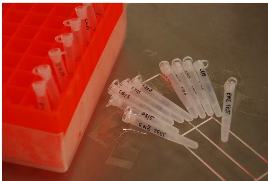
Figure 2.2: Microtubes containing plasmid samples prepared for the irradiation on HIMAC.
