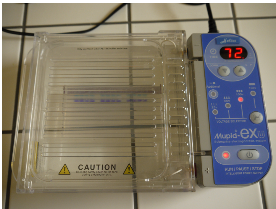
Figure 2.3: Agarose gel electrophoresis horizontal apparatus used in this study. The gel is placed in the buffer filled tank and electrical field is applied. The blue lines indicate the position of the migrating molecules.
