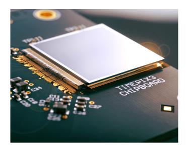
Figure 4.21: The Timepix3 Si detection region. The sensor consists of  $256 \times 256$  pixels with a pixel size of  $55 \times 55 \ \mu\text{m}^2$  and it is bump-bonded onto the Timepix3 readout ASIC below [122].
