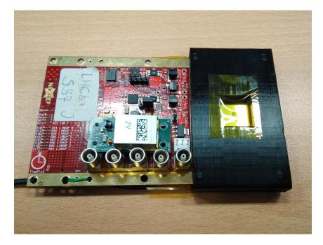
Figure 4.20: Timepix3 chipboard. The chip is covered with aluminium foil (to ensure an electric contact for biasing) with a hole that was cut off for experiments with lasers at Nikhef. The black plastic around the chip serves as a screen against stray light, the yellow kapton tape is to keep the chip clean and to ensure good transmission of X-ray photons.
