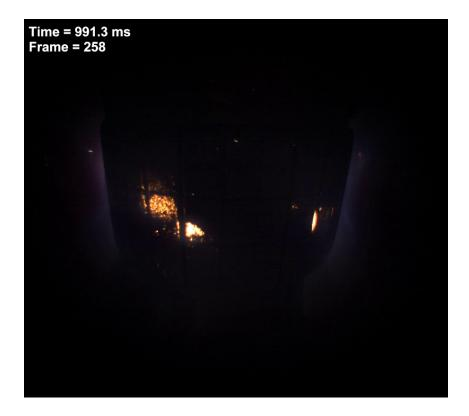
Figure 5.21: Shot 20056, tiles of the tokamak limiter hit by REs. Snapshot in the optical region using the camera Photron Mini UX100. The camera framerate is 6.25 kfps.
