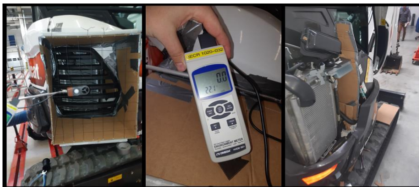
Figure 32 Measuring device, Grille separated to sections, measuring device and blocked air passages
