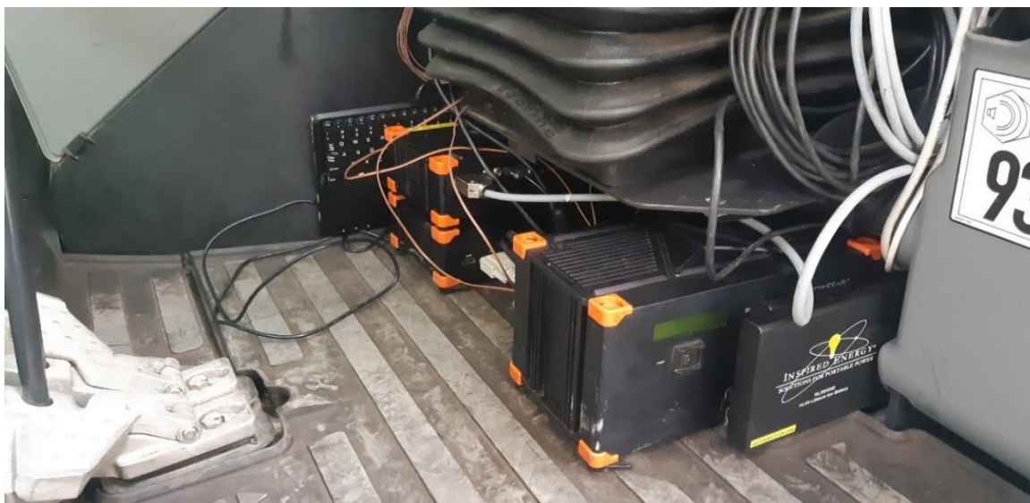
Figure 64 Data acquisition system packed under the operator seat, next to the keyboard the DEWesoft Sirius and Krypton units can be seen, on the right side there is an energy source
