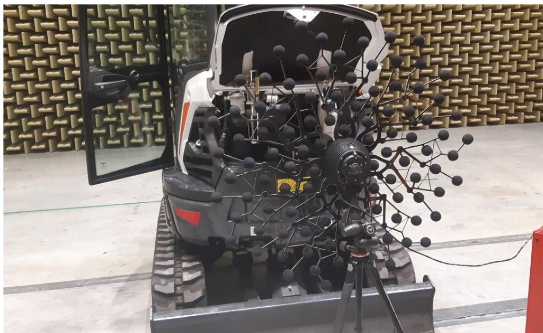
Figure 13 Noise camera measuring noise sources in the engine bay of the 2-3 tonne excavator
