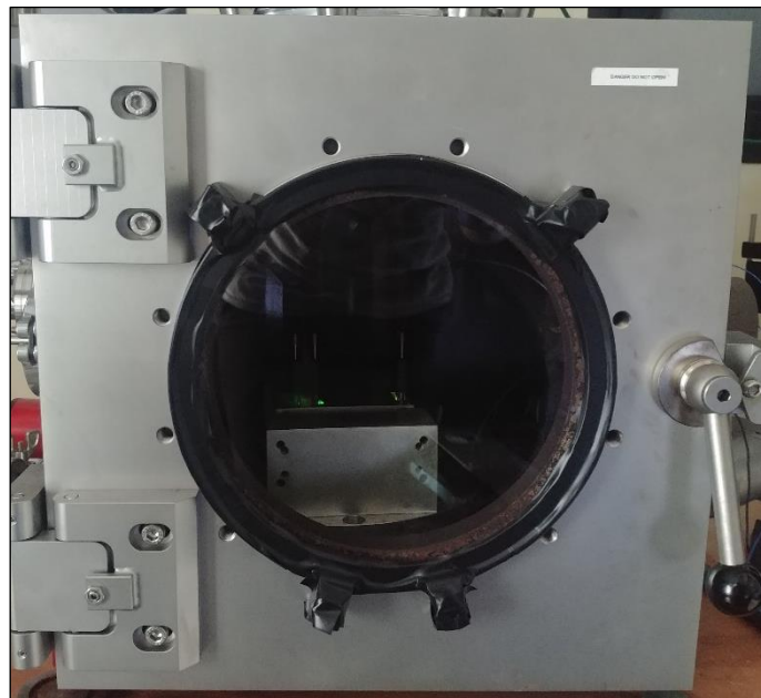
Figure 31: The vacuum chamber used to test the I2T5
