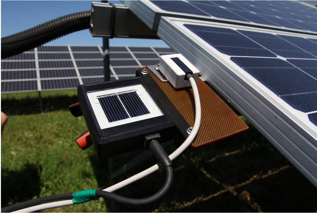
Figure 20: Sensors for measuring temperature and radiation intensity
