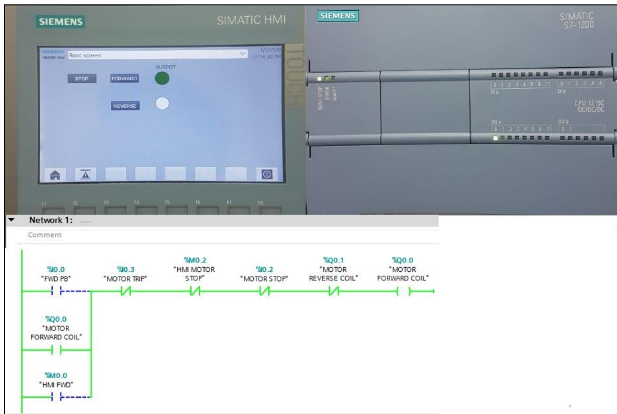
Figure 45: Online monitoring In TIA portal with PLC and HMI screen
