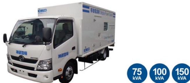
Obr. 8: Low-voltage Mobile Power Station [5]
