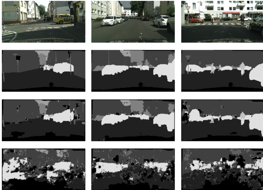
Figure 3.5: Semantic segmentation of sample images (256x512) from the Cityscapes dataset [3]. From top to bottom: input image, ground truth, output from trained model, output from quantized model. The last two rows demonstrate the accuracy loss of TensorRT we observed.
