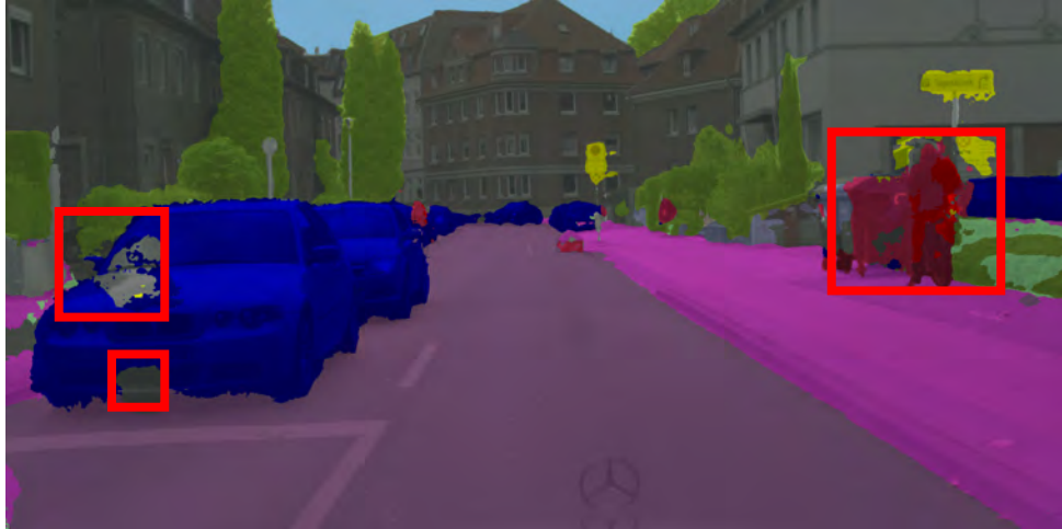
Figure 5.5: Failure of class prediction by networks utilizing LCMC and depth context, caused by anomalies in the depth image.
