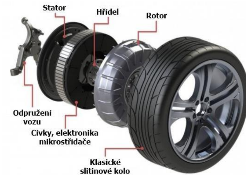
Obr. 6: Schéma motoru v kole [8]
