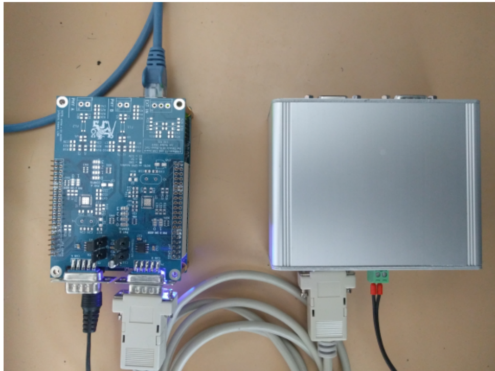
Figure 5.2: Control module (on the left) connected to one of the CAN Gateways (Gateway data interfaces are disconnected)
