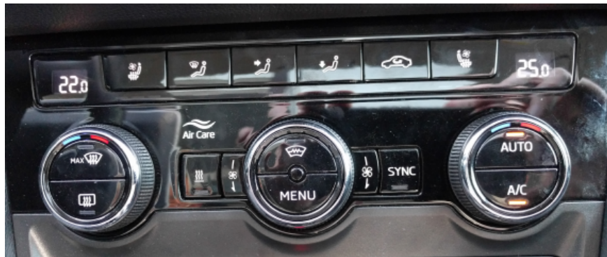
Figure 1.1: Control panel of Climate unit
