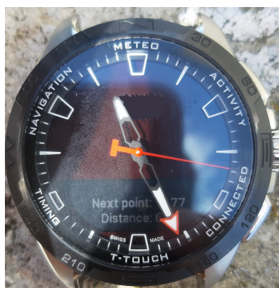
Figure 4.4: Photo of the watch displaying the actual take me home information - the number of points, the distance and the watch hand point to the direction of this point. Source: own work.
