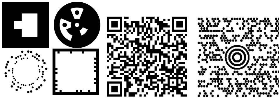
(a) : Frame (fiducial) markers can vary depending on the SDK, here it is (left to right, top to bottom): AR-ToolKit, InterSense, RUNE-tag-129 and Vuforia (ID 0)
