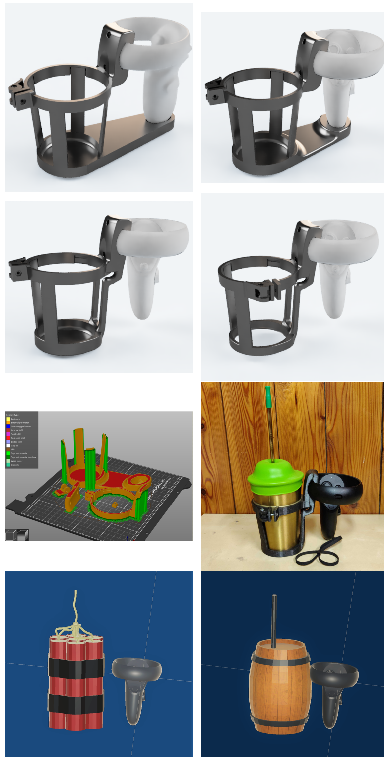
Figure 5.5: Last few 3D model iterations over the cup holder, one of the 3D print previews, final model with cup, controller, straw and rubber tip and 2 in-game verions of the cup
