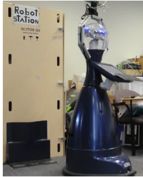
Figure 9: WhyCon markers as letter o in the “Robot station” sign to support docking into a charging station
