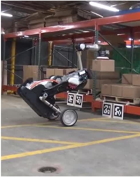
Figure 8: AprilTag markers as package and rack labels for warehouse robot
