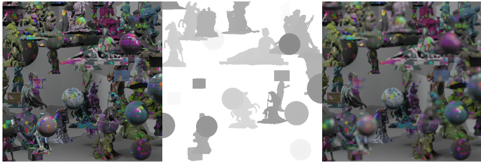
Figure 2.8: The DeepFocus dataset [36] contains images rendered using rasterization together with depth maps and corresponding images with accurately simulated defocus blur.
