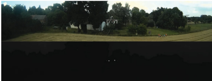
Figure 3.1: Comparison between the visible and UV camera footage from UVDAR, collected during an experiment. The UV image is significantly easier to process to retrieve information on the observed MAV. [12, p. 2638]
