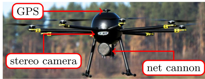
Figure 3.6: AAIS MAV platform, which was used in experiments with CNN-based MAV-detection [22, p. 3407]
