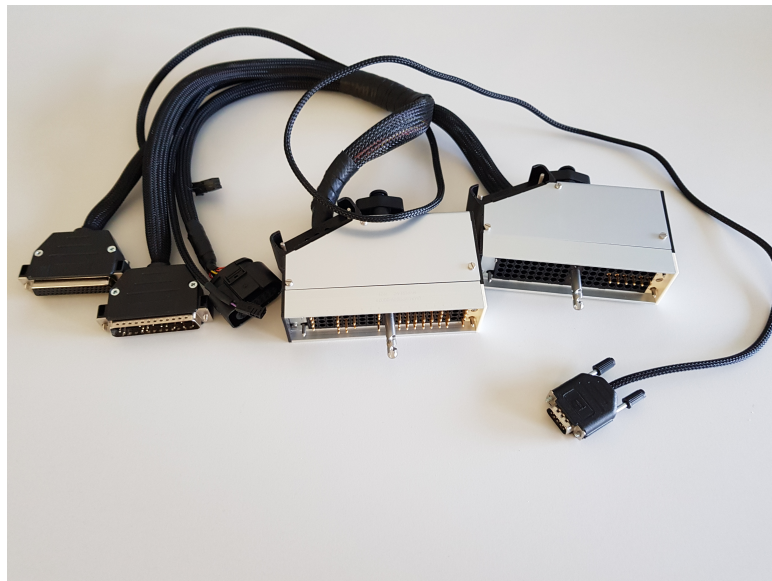
Figure 5.2: Created cable harness.
