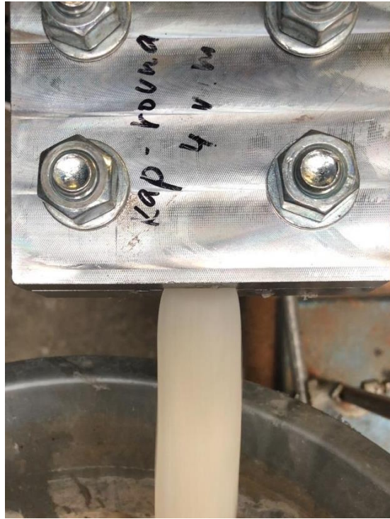
Figure 23: Collagen extrusion through capillary slit rheometer
