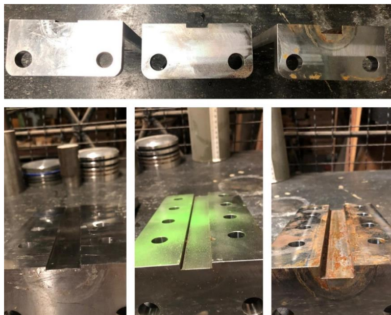
Figure 22: Slit dies used in the extrusion capillary rheometer
