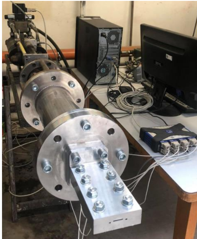
Figure 21: Capillary rheometer used for experimental measurements
