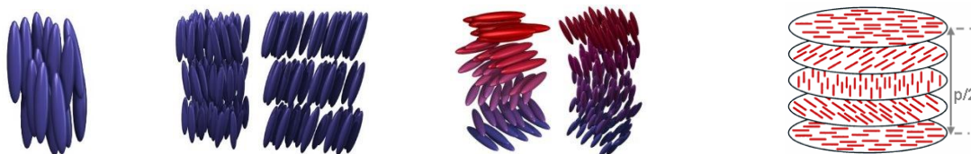
Figure 1.4 Schematics of molecular alignment in the nematic, smectic, chiral and columnar phases respectively. (Andrienko, 2018).
