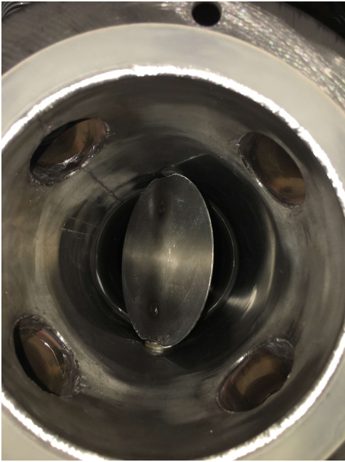
Figure 8.6: Rotated valve from configuration A may have impeded the correct measurement of air flow
