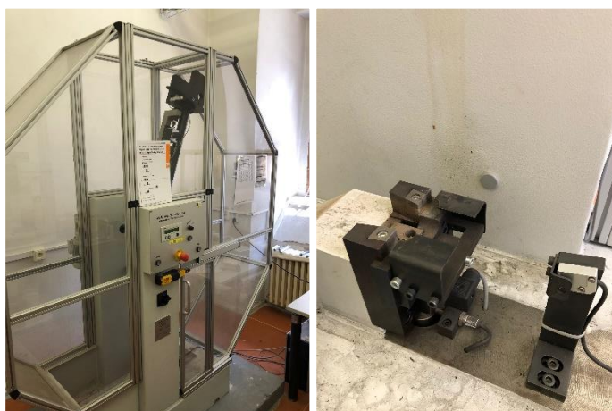
Obr. 29 – Impact Tester PH 300 – S Version CHY.
