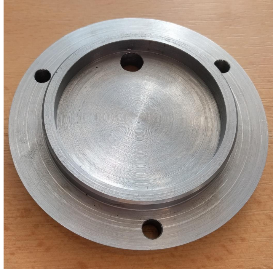
Annex XI – Manufactured new cover for the old headform impactor.
