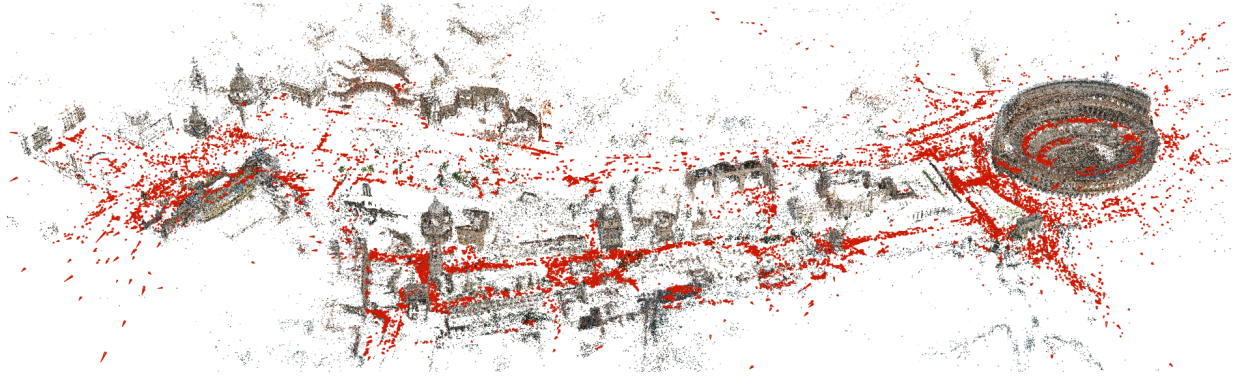
Figure 3.6: Sparse model of central Rome using 21K photos produced by COLMAP’s SfM pipeline, taken from the software’s website.
