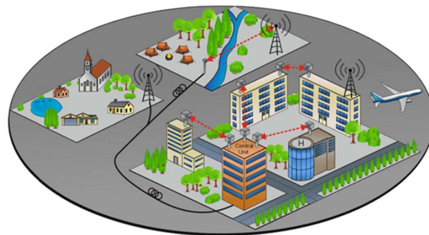
Fig. 1. Example of RoF and RoFSO scenario adopting C-RAN architecture.
