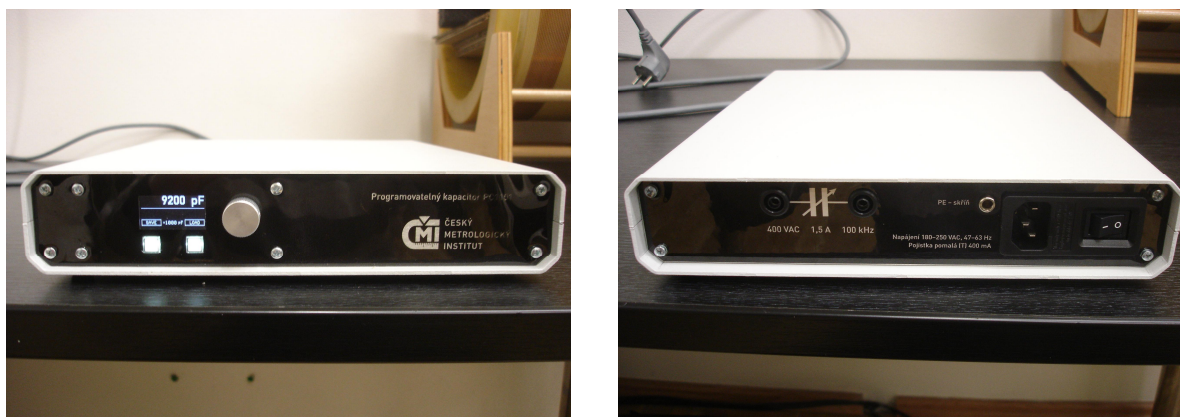
Fig. 32 Programmable capacitor array PC1101.
