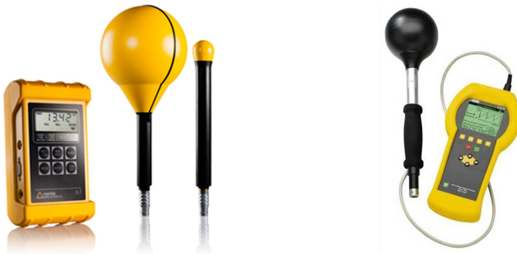
Fig. 47 A magnetic field analyser with an ELT 400 3-axis coil probe (left) and C.A. 42 (right). Pictures taken from the Narda Safety Test Solutions (ELT 400) website and from Chauvin Arnaud website (C.A. 42).
