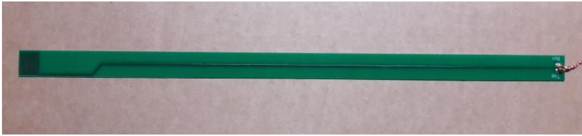
Fig. 38 The SC1L_30 single-layer PCB search coil.
