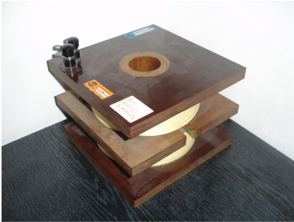
Fig. 17 Helmholtz-type solenoid standard No. 051.
