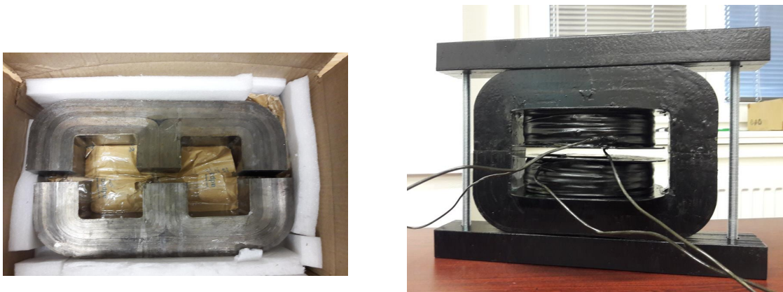
Fig. 74 a) Core made from Metglas 2605SA1, b) the AC electromagnet made from Metglas 2605SA1 material.
