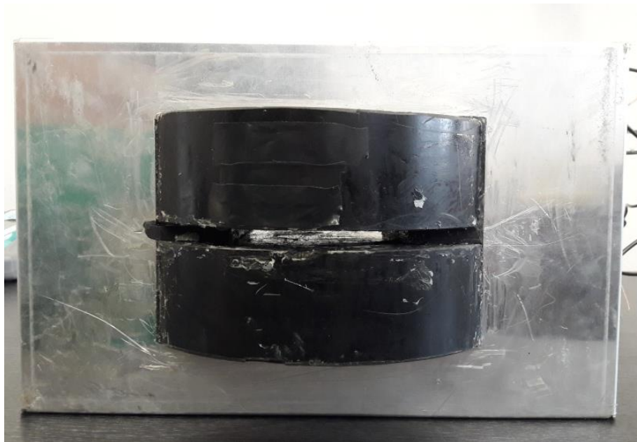
Fig. 67 The AC electromagnet with a UNICORE core.
