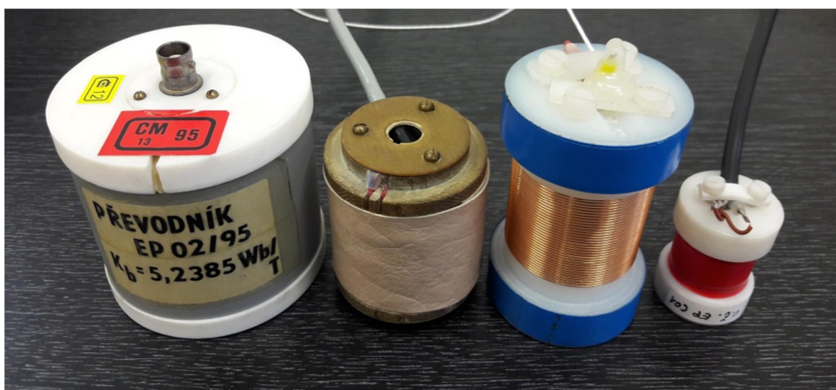
Fig. 25 Special search coils (from left): EP 02/95, K_{II} , EP 01/00 and EP 601.
