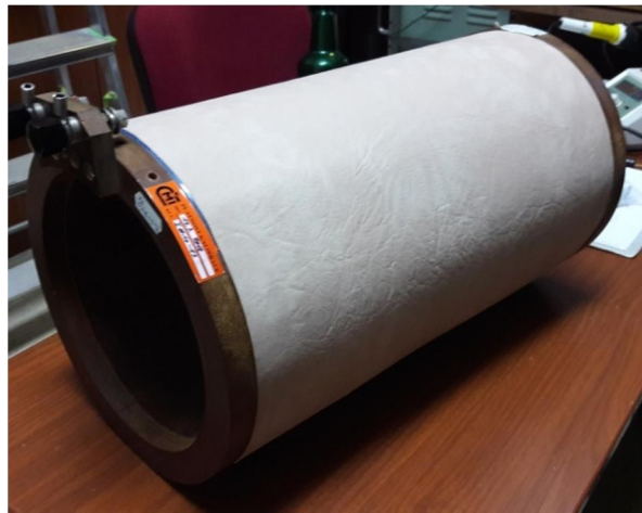
Fig. 21 Garrett solenoid standard No. 8003.
