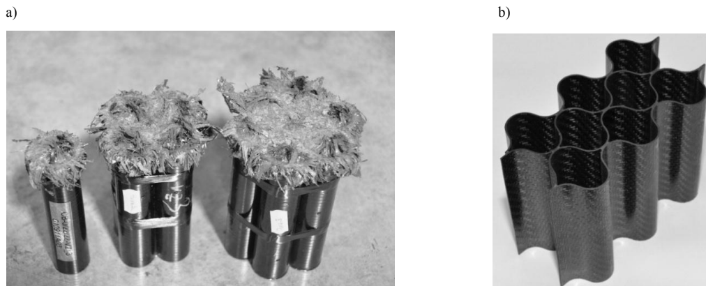
Fig. 1. (a) Individual tubes and bundles of 4 and 7 tubes (after the impact test); (b) Deformation element box made from four connected corrugated sheets (before impact test).
