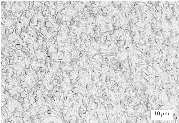
FIGURE 11: SEM micrograph showing the microstructure of solid state hardened zone.
